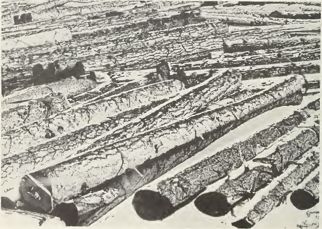
Figure 15. --Logs banded together for storage in a log pond.
